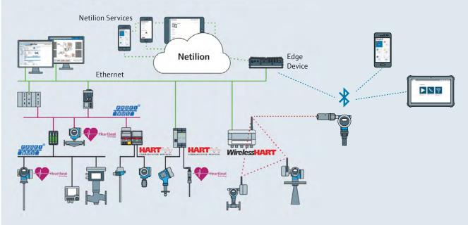
Example of the different possible communications networks (HART, Profibus, Ethernet IP, WirelessHART, Bluetooth, Cloud)
