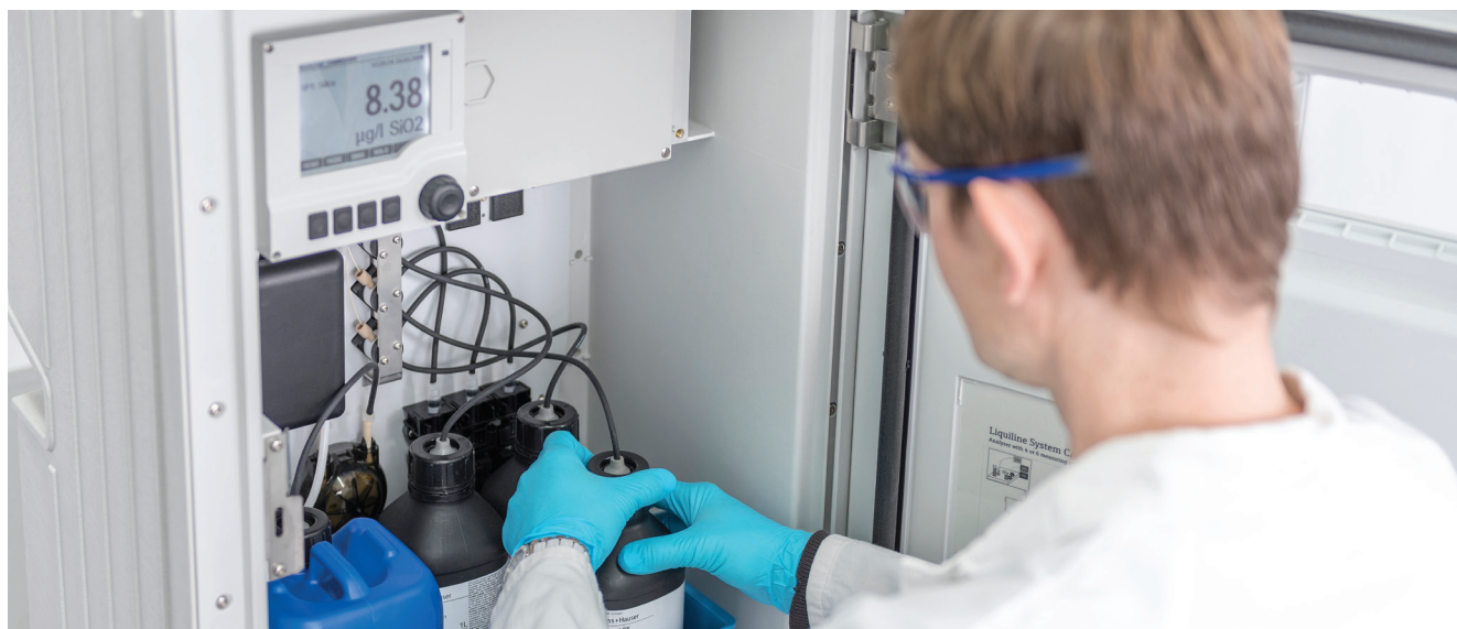
Endress+Hauser's Liquiline System CA80SI silica analyzer
