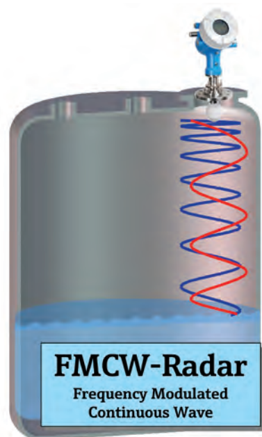
FIGURE 2. FMCW radar sends a continuous wave that reflects off the surface and returns to the antenna. The shift in frequency determines the level in the tank.
