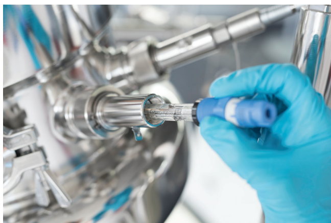
Figure 2: Glass pH sensors are fragile. Handle carefully.
